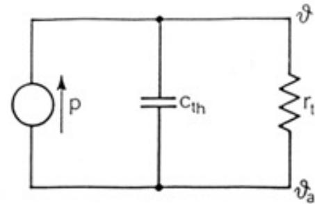
Heat release from a **bare conductor** in air heated by thermal power  $p$  and its equivalent thermal circuit.
