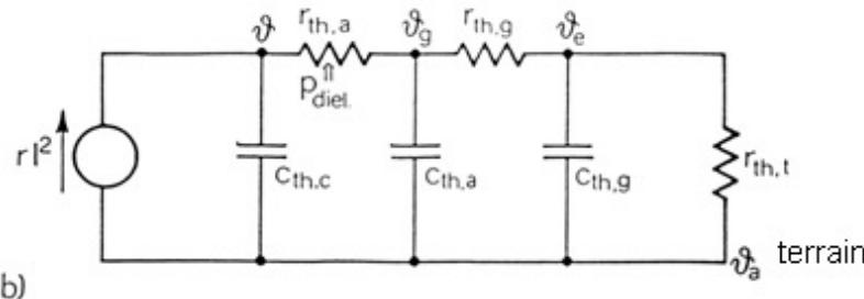
Schematic representation of heat transfer for a **single-core cable with insulation laid in homogeneous soil** (a) and its equivalent thermal circuit (b).
