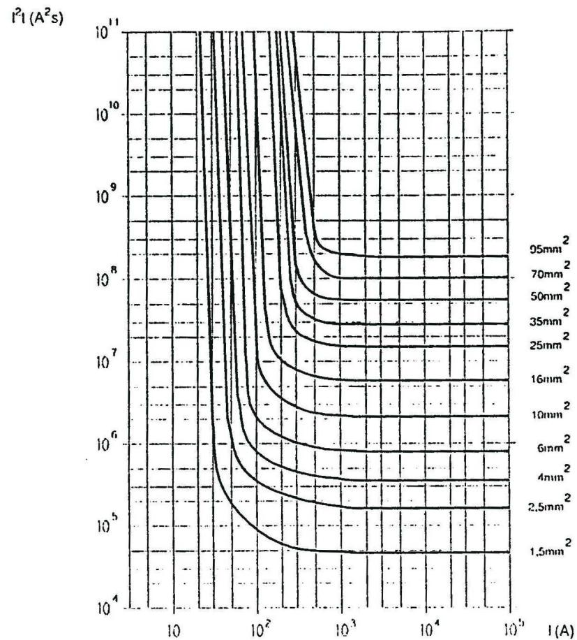
Joule integral (or specific energy) curves as a function of cable current (EPR, copper, three-core, laid in air)
