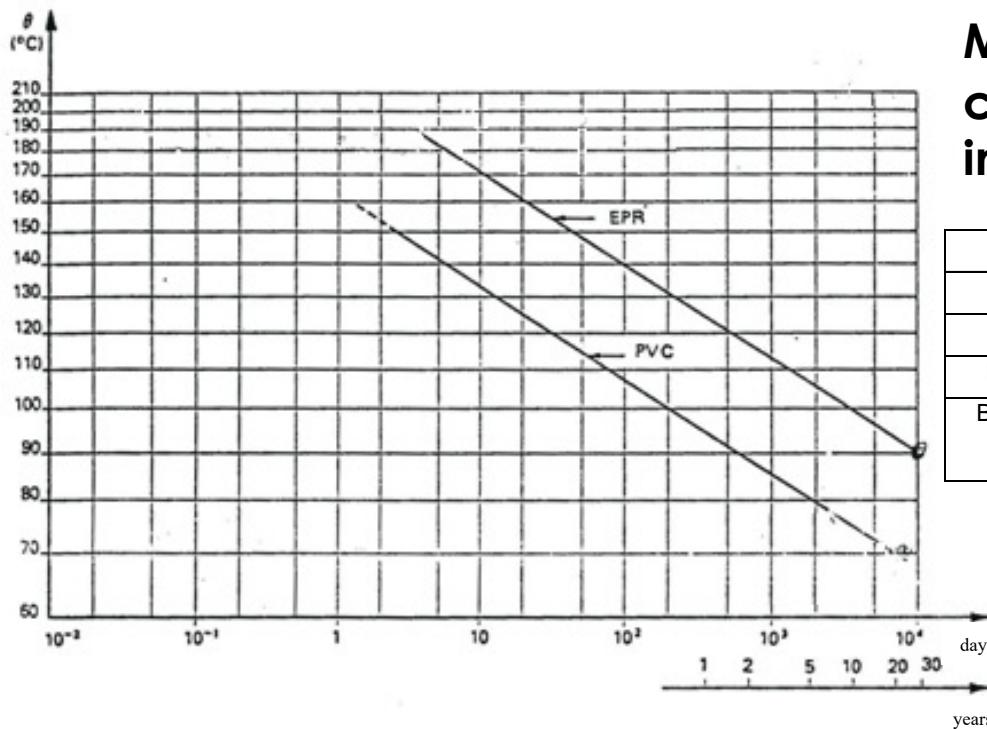
**Maximum service temperatures  $\theta_s$  of conductors for cables with different insulation materials**
